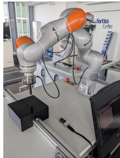
Fig. 3: Demonstrator setup with a KUKA IIWA 7 R800 robot and attached cylindrical peg, black target box with hole, and Kapoho Bay containing two Loihi chips (on the tabletop).
