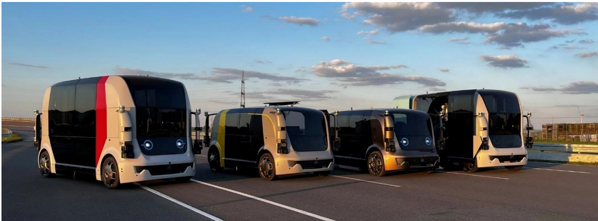
Fig. 1 The UNICAR agil research vehicles. From left to right: autoSHUTTLE for public transportation, autoTAXI for individual business rides, autoELF as a private vehicle and autoCARGO for the delivery of goods. © ika
