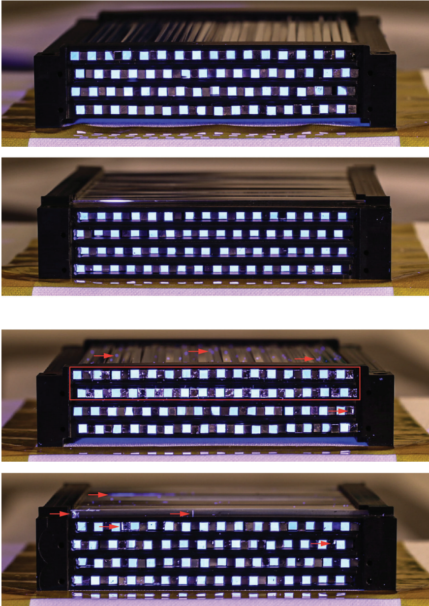
Figure 8.14: Assembled modules prior to installation of the SiPM arrays. The fibers in the upper pictures are of good quality; the coating of those in the lower pictures shows substantial signs of abrasion, scratching, and flaking (exemplarily marked in red).
