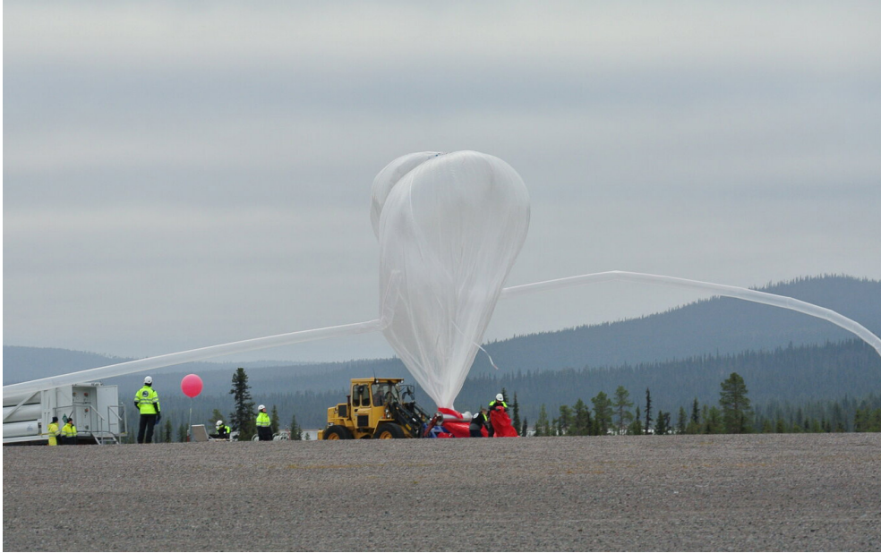
Figure 6.20: The BEXUS 18 stratospheric balloon shortly before launch from Esrange Space Center in Kiruna, Sweden. It reached an altitude of about 27 km and stayed aloft for a little over three hours. Image credit: ESA.
