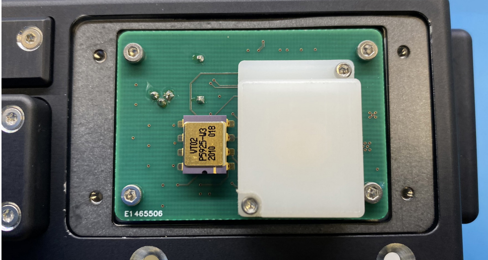
Figure 10.7: Accommodation of the two RADFETs in the housing of the RadMap Telescope. One VT02 is visible on the left, the other is hidden below a shield made of white POM.
