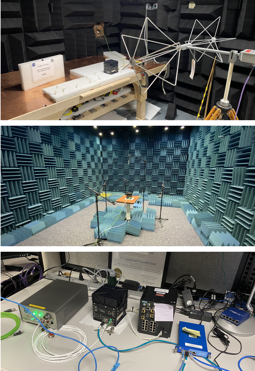
Figure 10.29: The RadMap Telescope during EMI (top), acoustic (center), and JSL (bottom) testing at NASA's Johnson Space Center.
