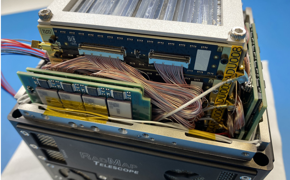
Figure 12.7: Photo of the RadMap Telescope’s ADU after integration, illustrating how we needed to squeeze the cables between the detector and the PCB assemblies of the read-out electronics
