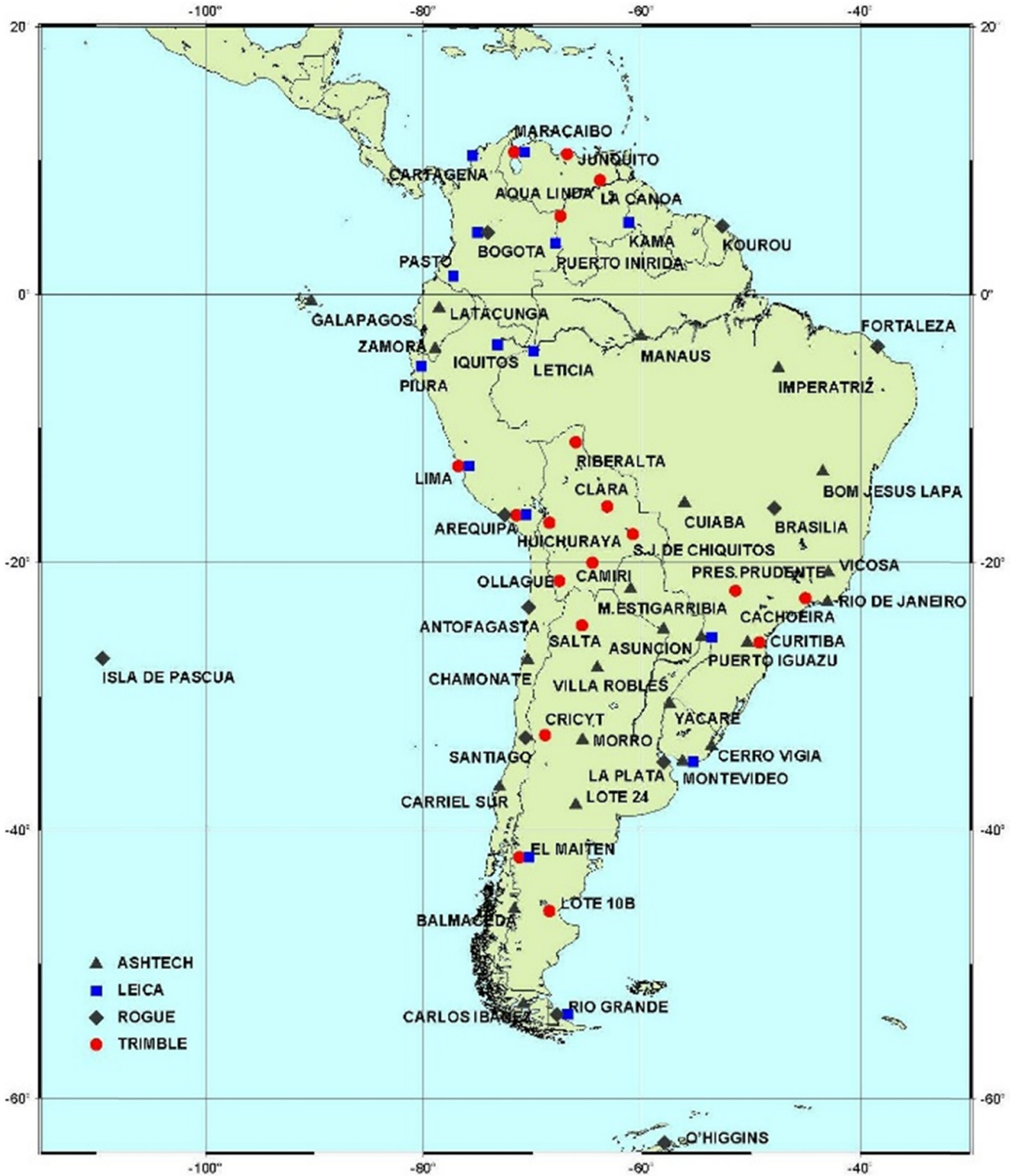
Figure 3: SIRGAS 1995 reference frame with four employed receiver types.
