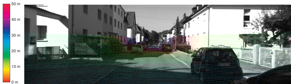
Figure 4.15: LiDAR point cloud projected onto a grayscale image from the KITTI Odometry dataset [42]. Each point is colored according to its distance from the sensor.
