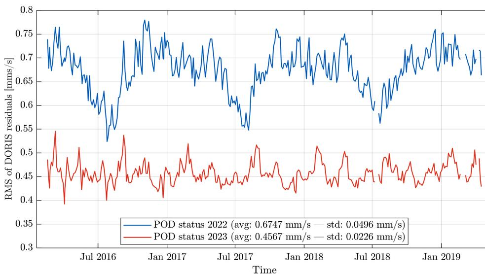
**Figure 1.3:** Arc-wise RMS of DORIS observation residuals for Jason-3 before and after the implementations made in 2023.
