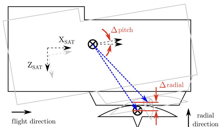
**Figure 1.7:** A change in the pitch angle of an altimeter satellite results in a change of the altimeter phase center in radial direction and can cause an erroneous estimate of the sea surface height.
