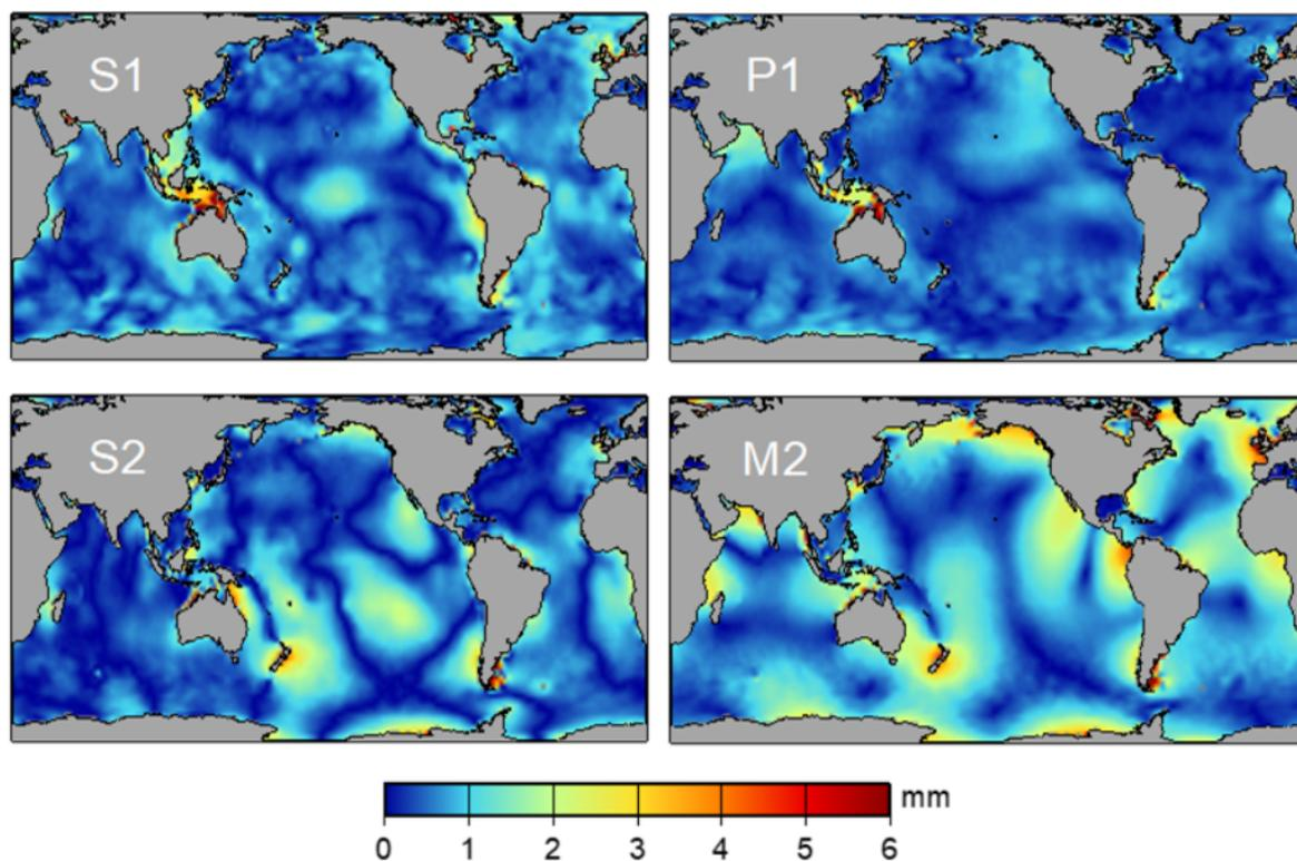
**Figure 2.1:** Results of harmonic analysis on gridded DAC for four of the major tidal constituents.
