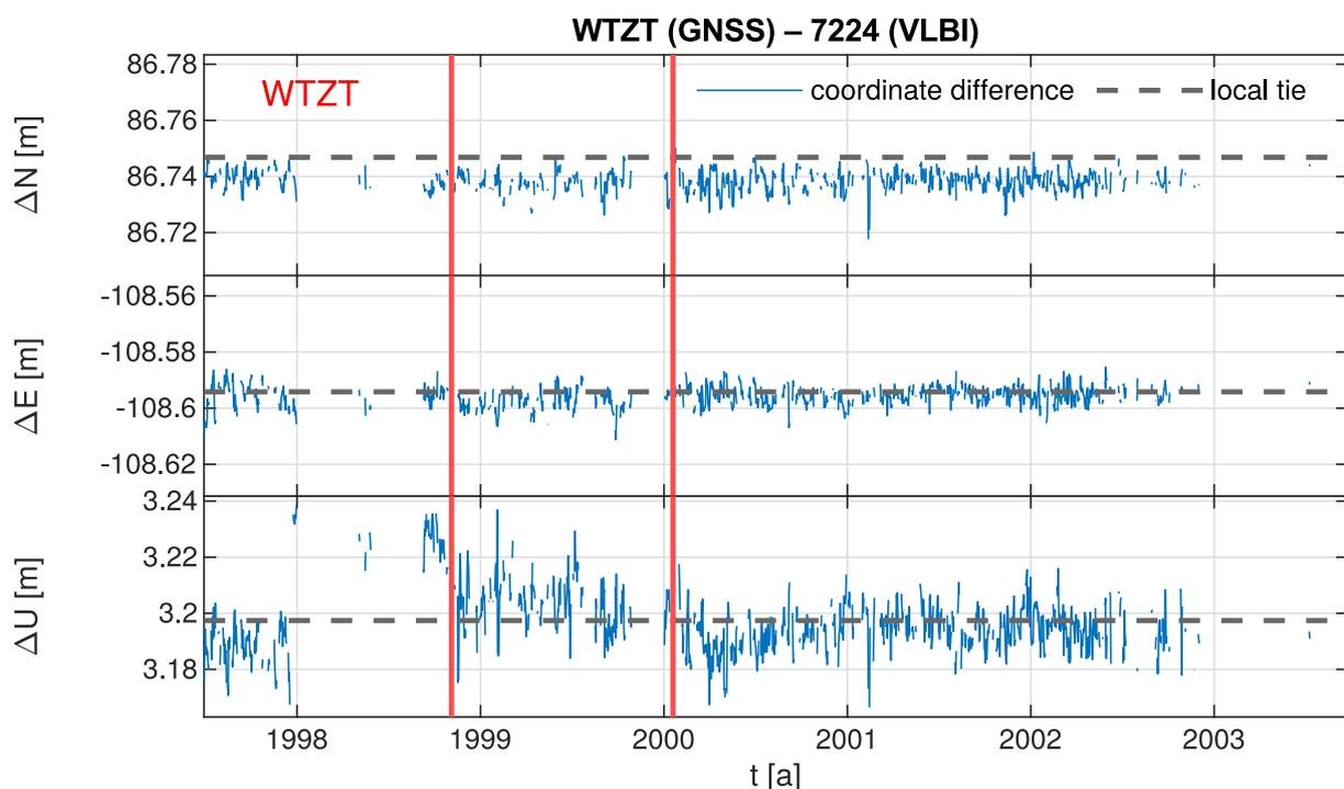
**Figure 1.14:** Difference of the position time series of GOW's GNSS station (WTZT) and VLBI station (WTZ) plotted relative to the local tie, i.e. the coordinate difference between both stations from local survey. Red vertical lines mark GNSS antenna changes. They are reflected by artificial jumps in the time series.
