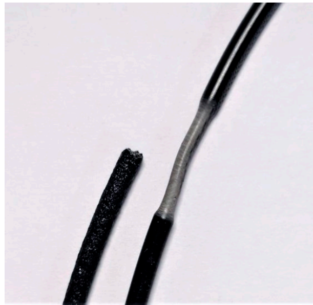
Figure 4. Comparison of a brittle (left, Nylon + GF) and a ductile (right, ABS) filament failure.
