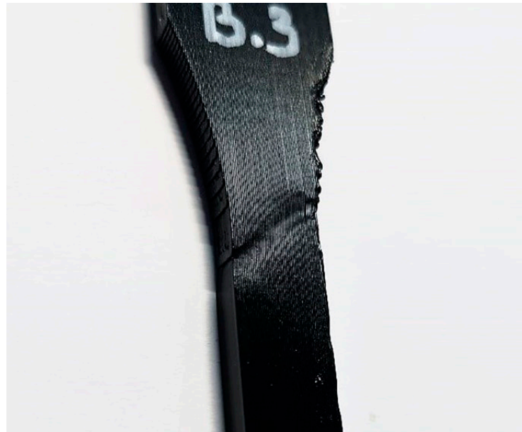
Figure 10. Necking in the taper area of specimen B.3.
