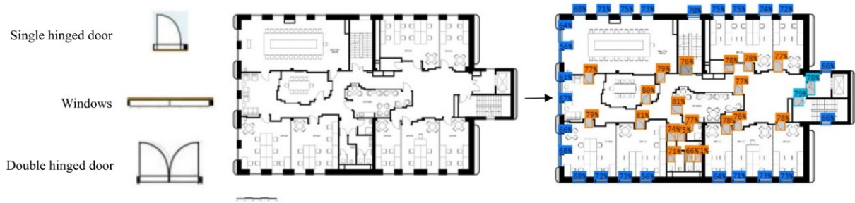
Figure 4: The three opening elements to train the object detection model (on the left) and an example of opening detection (on the right)
