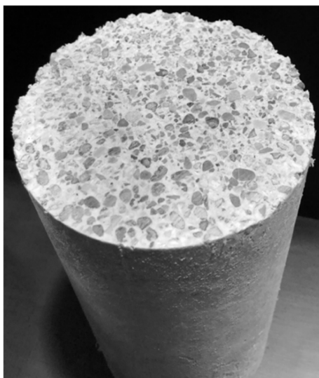
Fig. 8. Test specimen of foam-injected fGr with cut end face H/D = 2 .
