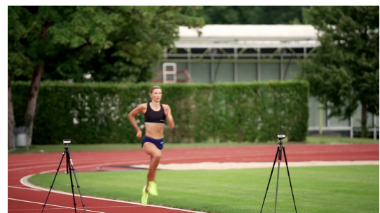
Figure 3.7 Timing Gate usage in running. The elapsed time until an athlete reaches the precisely marked position on the track is captured by TGs that are placed on tripods. The signals of the TGs are forwarded wirelessly to a central stopwatch.
