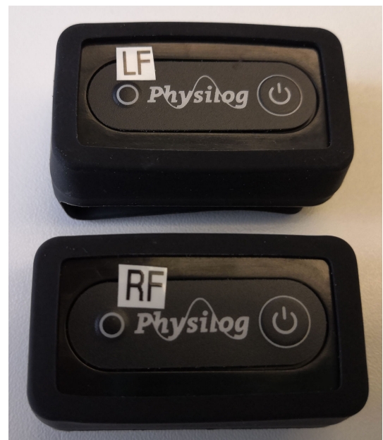
Figure 3.5 Inertial Measurement Units for running. The labeling was done for the left foot (LF) and the right foot (RF). The data output of both sensors is the same. The attachment is done in the manufacturer's rubber case.
