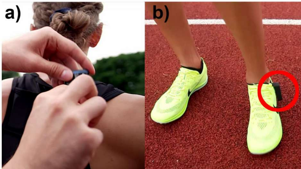
Figure 1: GPS receiver attachment location (a) and IMU sensor attachment location at both shoes (b).
