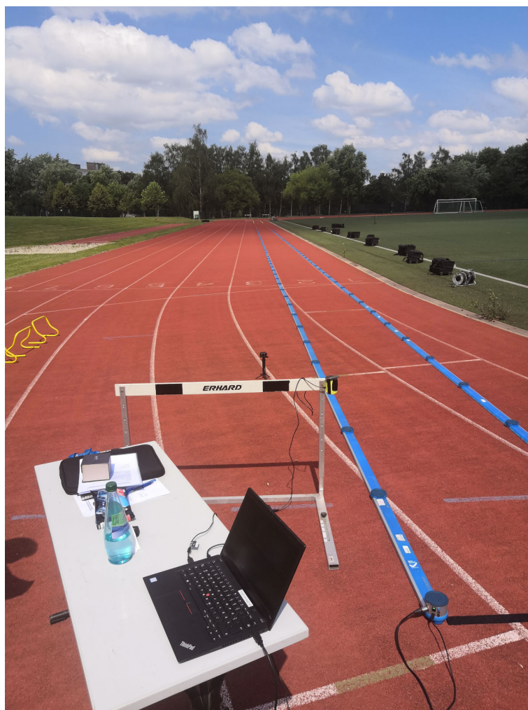
Figure 3.8 Measurement setup of Optogait at a running track. OptoGait strips are placed on the track over the course of 50 meters for tracking the first half of a 100-meter sprint.
