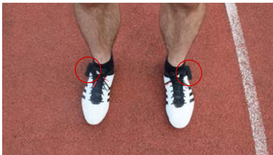
Figure 1. Sprint shoes with IMUs attached to the ankles (red circles).
