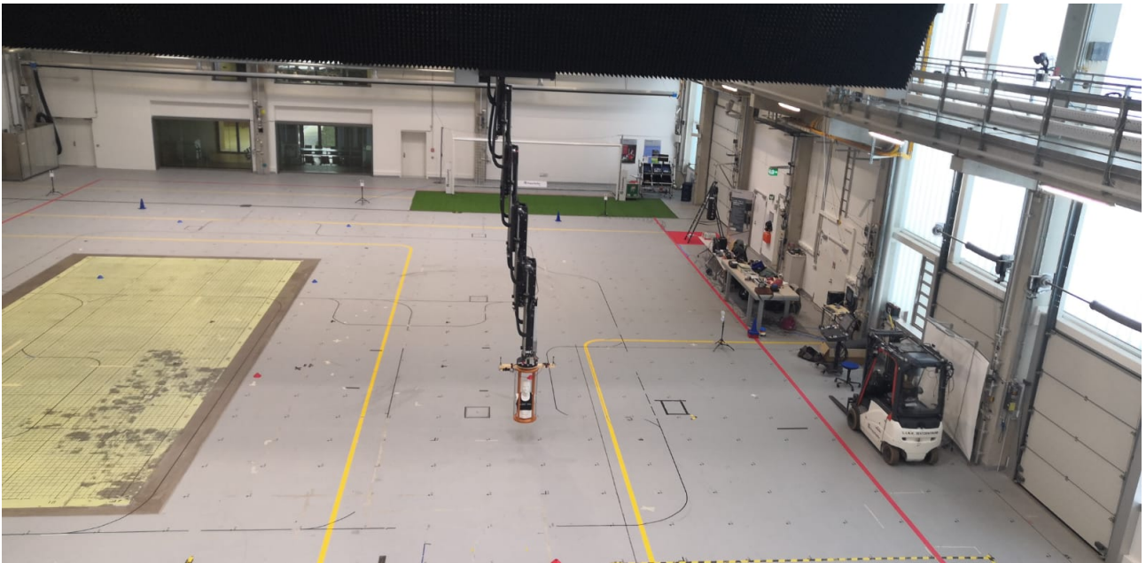
Figure 4.1 Measurement hall of the study. As the objectives of the study required a precise infrared motion-capturing system, an indoor facility was used. The marks at the ground and the electronic placement arm were used for precise position tracking.
