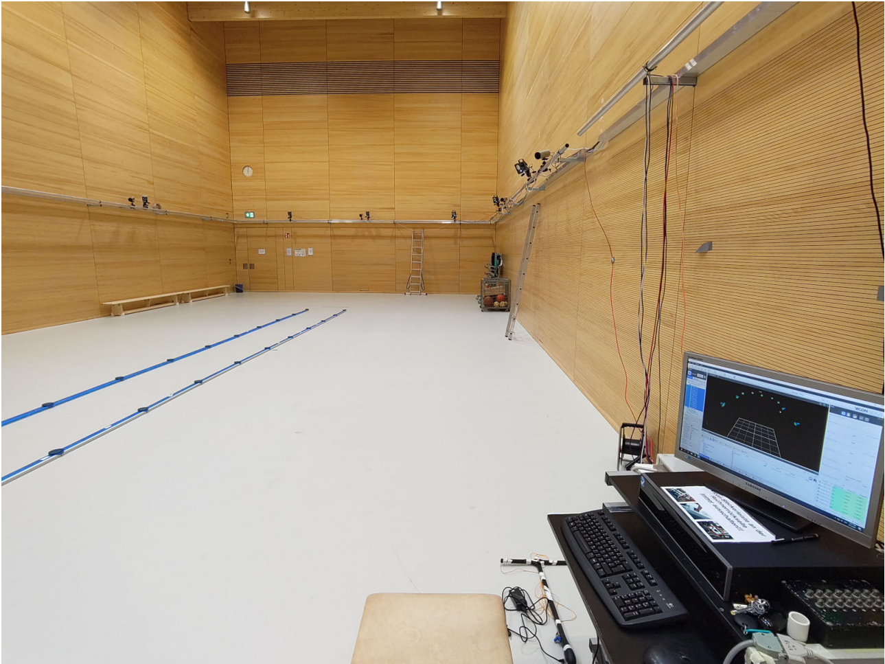
Figure 3.6 Measurement systems at the university's diagnostics hall. An infrared motion-capturing system (Vicon) is mounted on the rail system around the hall. OptoGait strips (blue) are placed on the floor.
