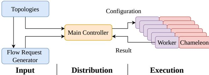
Fig. 1: Data flow overview for running the tests to get the performance of networks
