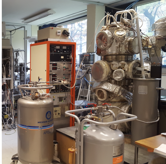
Figure 6.2: A picture of the tungsten evaporation system at the Max Planck Institute for Physics in Munich. The ultra high vacuum chamber is shown, covered with the heating blankets, which were used for the system bake out in the past.
