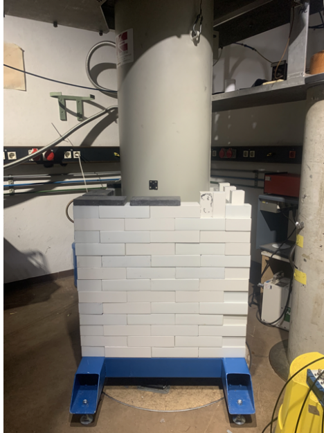
Figure 7.11: Photo of Cryo 2 closed and surrounded by a 10 cm thick lead shield in the above-ground facility of the Max Planck Institute for Physics in Munich. The lead shield was borrowed from the COSINUS group at the Max Planck Institute for Physics. The picture was taken during the data taking of the first measurement of the first doubleTES prototype.
