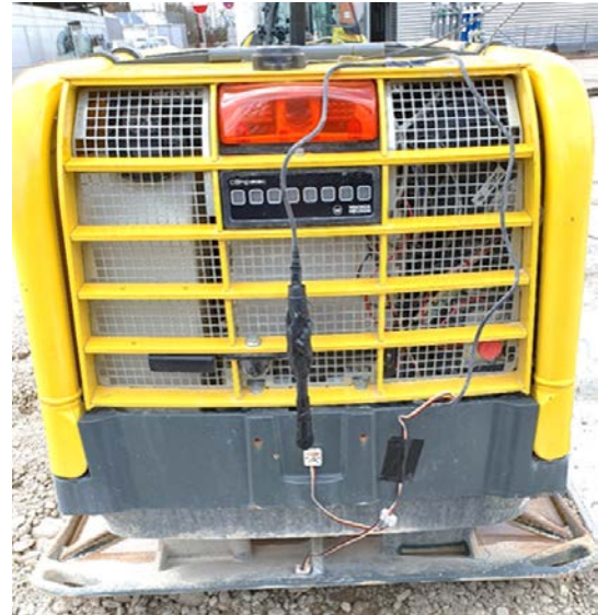
Figure 3: Sensor placement on the vibratory plate
