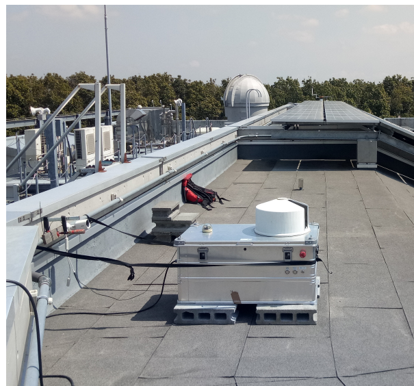
Figure 1. The figure shows the TS in Tsukuba, Japan whilst measuring. The enclosure including its measurement dome, developed by TU Munich, can be seen in the foreground. The white hemisphere in the background is the TCCON dome.
