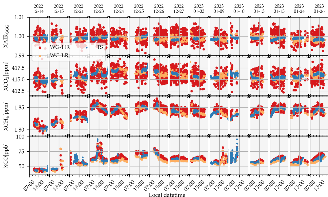
Figure 12. XAIR and XGas data of the Wollongong campaign. For all species, the overall agreement is good. It is interesting to see that the WG-HR data are much noisier than the WG-LR data. This is discussed in Sect. 7.1. Compared to the Tsukuba data, the difference of the XCO LR and HR data is smaller. This is probably due to better a priori profiles of the less urban area of Wollongong compared with Tsukuba. The subscript “GGG” at XAIR indicates that the XAIR values of PROFFAST are inverted to be comparable with the GGG XAIR values.
