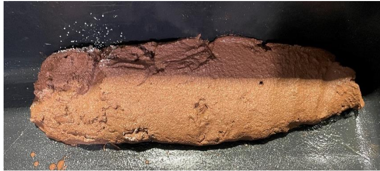
Figure 4-4: Sample extraction from the mixing zone: 435 mm in length, starting at 160 mm
