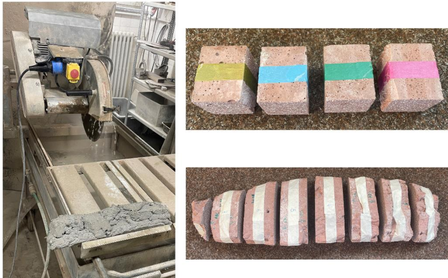
Figure 4-6: Left: Wet cutting of samples in cubic meters at Centrum Baustoffe und Materialprüfung; top right: Cut samples from the end product; bottom right: Cut samples from the mixing zone.
