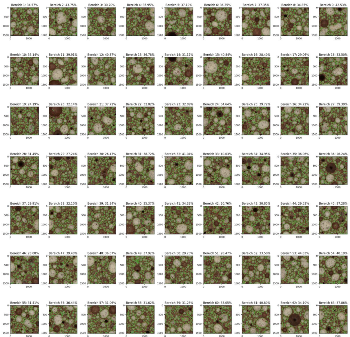
Figure 4-15: The micrograph is segmented into defined area units, and the Poraver content is calculated for each respective area unit.
