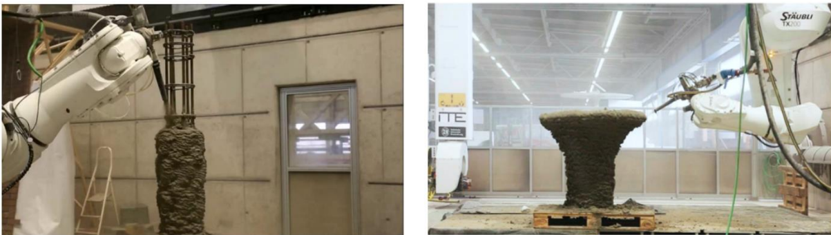
Figure 2-9: Left: SC3DP with substrate/reinforcement [Hei-2022]; Right: Free-formed SC3DP [Lu-2020]
