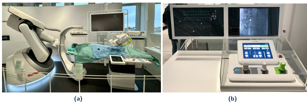
Fig. 5.14. Corindus system displayed at the Deutsches Museum in Munich. (a) Robotic C-arm fluoroscope and robotically navigated catheter manipulator, and (b) Master system from which the physician manipulates the remote catheter, featuring two screens displaying vitals and live fluoroscopic images, as well as controls for catheter manipulation.
