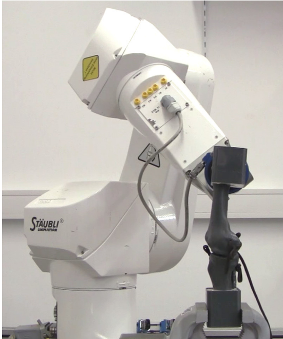
Figure 4.2 Test setup for the Multi-Force Control. The robot is attached to an additive manufactured replica of the human knee-joint constrained by tendons [8].
