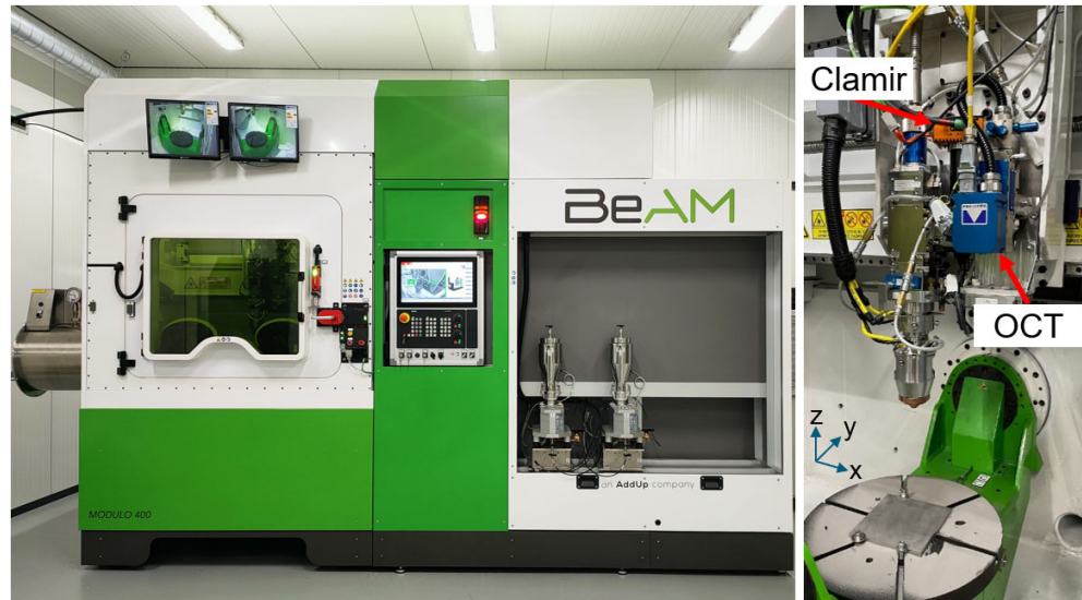
Figure 1. BeAM Modulo 400 machine (left) with the integrated sensor systems and machine coordinate system (right).
