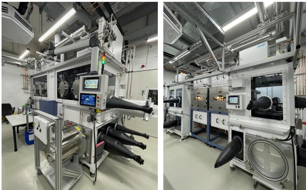
Figure 4-11: Photos of the machinery at *iwb* showing the microenvironments for the coater (right) and calender (left) machinery.
