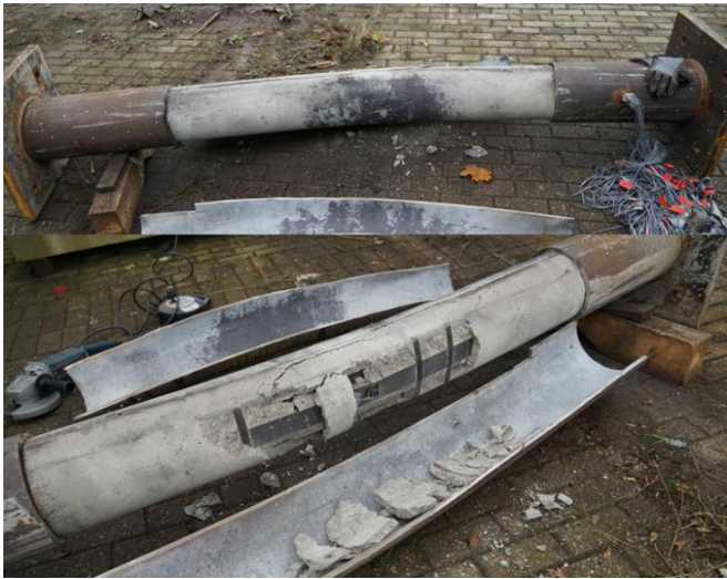
Figure 3-15 Concrete section in the compressive zone (top) and tensile zone (bottom) for KR-6.
