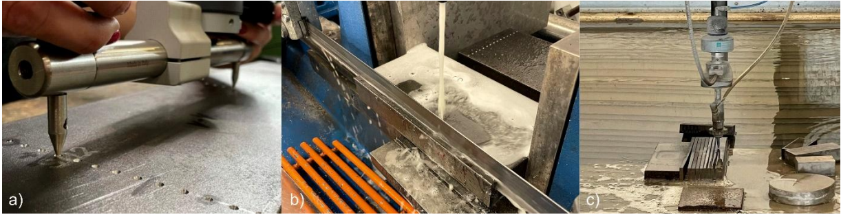
Figure 3-27 a) Strain measurement with deformer b) sawing of the segments and c) water jet cutting of the segments.
