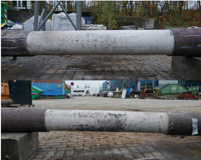
Figure 3-14 Concrete section after testing with tensile zone (top) and compressive zone (bottom).
