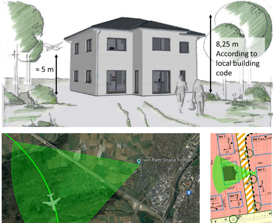
Figure 64: View from Köngen towards the flight path of the RNP routing. The observer is standing on Erwin-Rath Straße (green cross). Looking to the southwest (green circle segment), the aircraft on the B-D variants appears at the highest point at an angle of 27° from the horizon. For an airplane on variant A, the angle increases to about 31°. The top of the roof of the house (dark green) as seen from the opposite sidewalk appears at an angle of 42°. The aircraft is shown at the approximate position in the sky as seen by the observer, but is not to scale itself. This graphic was shown at the Köngen town council meeting on Oct 4, 2021. Source: own illustration.
