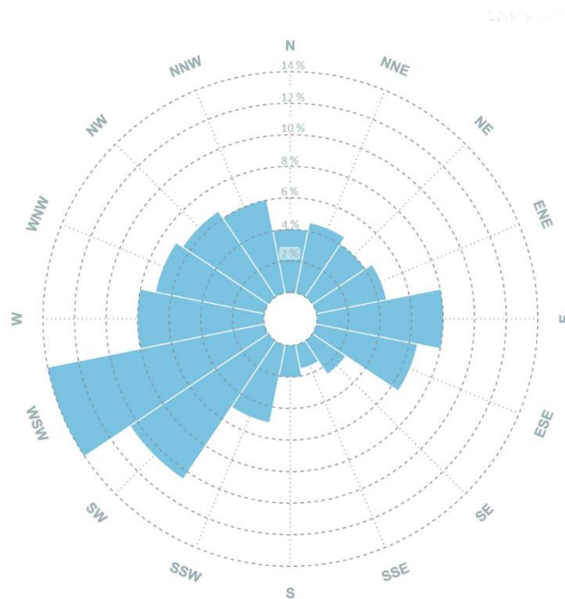
Figure 53: Average distribution of the wind direction in % at Stuttgart Airport between 1961 and 1980. Source: Amt für Umweltschutz Landeshauptstadt Stuttgart (n.d.).
