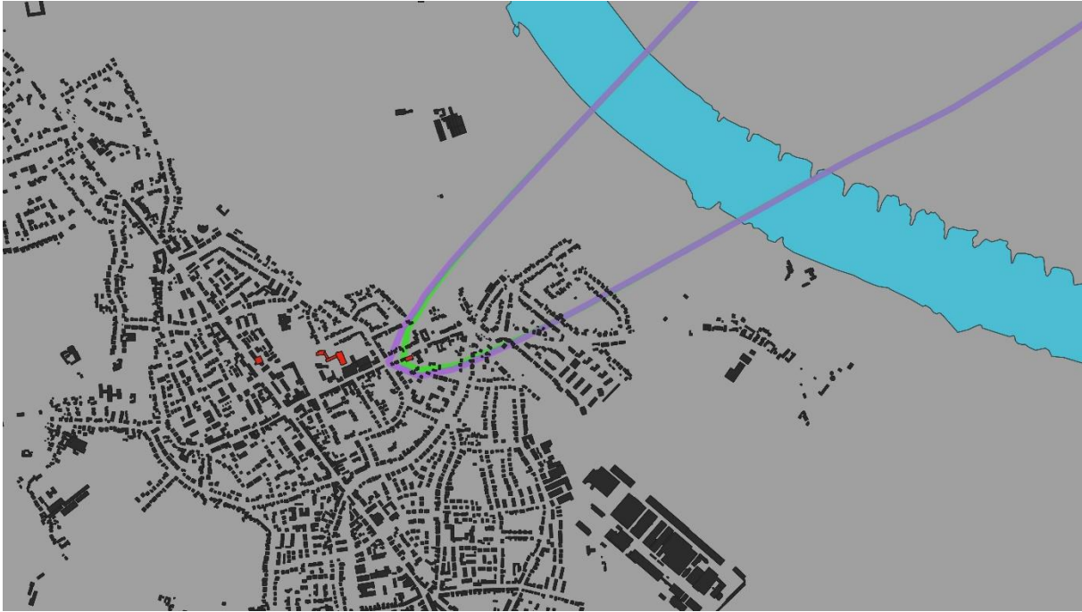
Figure 76: Noise contour for the aircraft mix accelerating at an altitude of 5500 ft. In comparison to the NADP 1 contour (green) no major differences are calculated.
