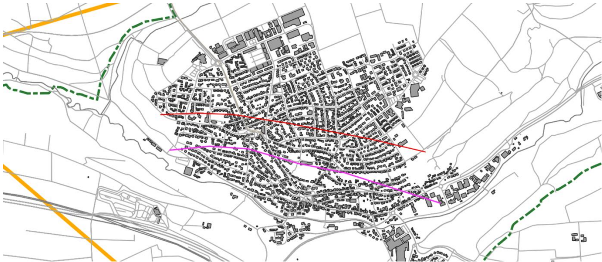
Figure 62: Denkendorf – Calculation of a neutral line defining noisier and quieter urban parts. Depicted are the lines of the initial variant A, and variant C, which was generated as a redesign. While the neutral line of variant A splits the town almost in the middle with a decrease in noise emission to the north of the line, the majority of the settlement area is receiving less noise through variant C. This graphic was shown at the Denkendorf town council meeting on Sep 20, 2021. Source: own illustration.
