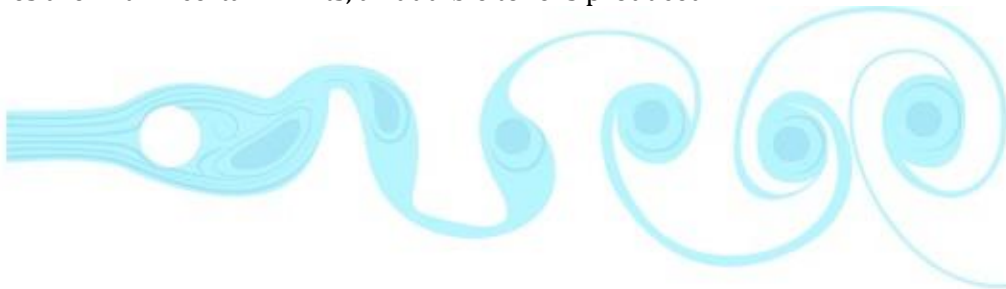
Figure 8: Illustration of sound creating eddies in the flow behind a cylindrical object. Source: Schade et al., 2022, p. 384.
