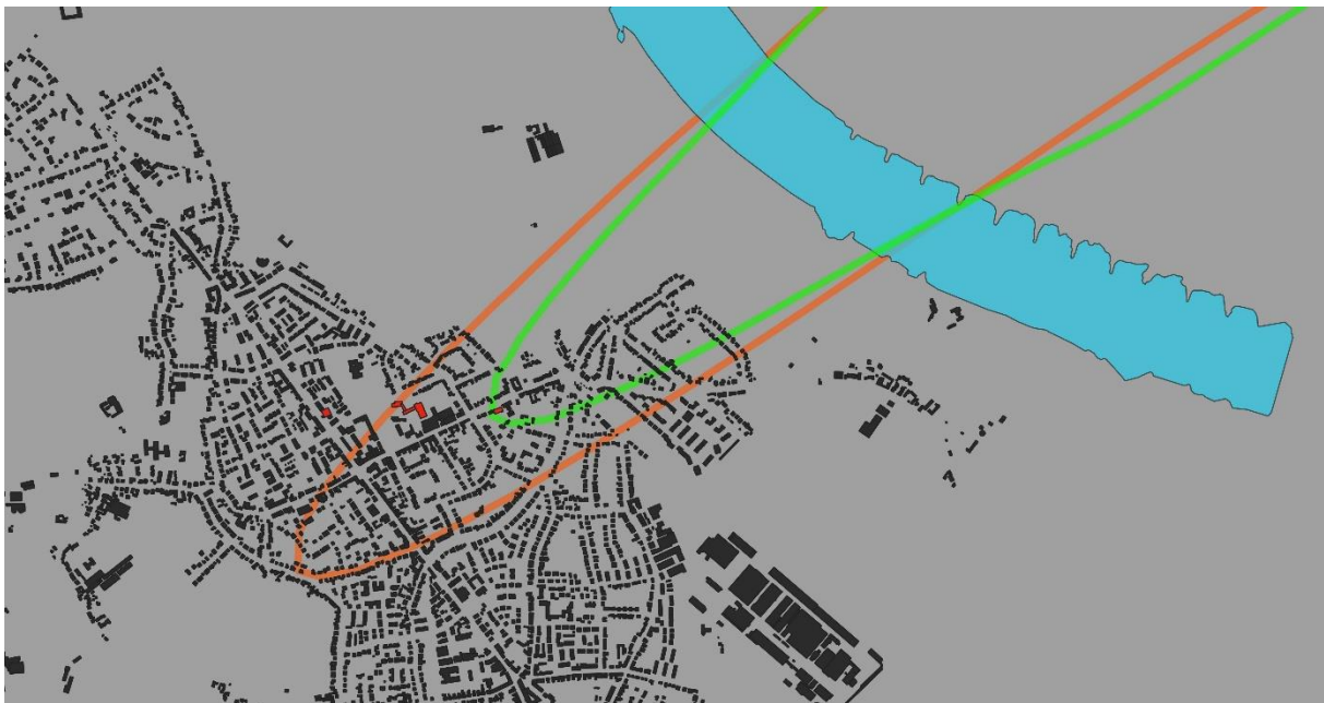
Figure 75: Result of solution one. 56,6 dB L_{eq} contours as calculated by Impact with the aircraft mix scenario, performing NADP 2 (red contour) and NADP 1 (green contour). The L_{eq} contours differ by around 900 m.
