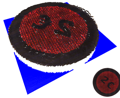
Figure 6. RGB-D point cloud of the validation coin fused by JBU.
