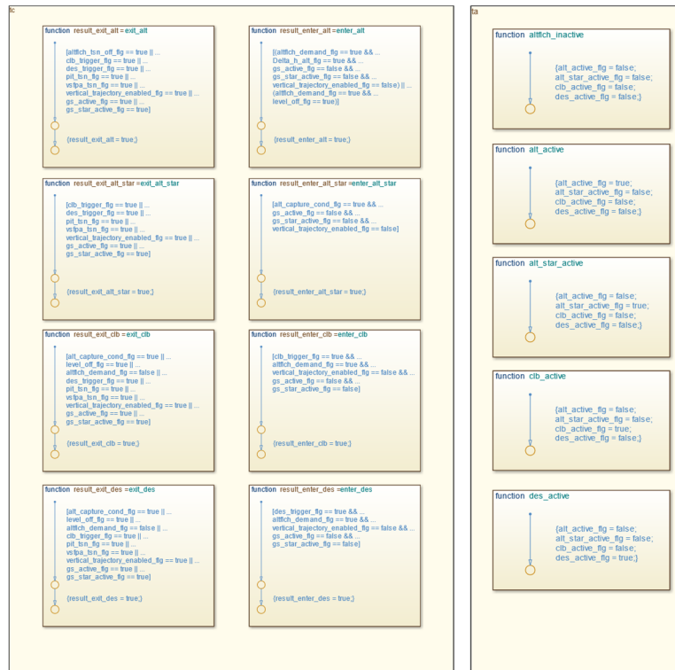
Figure 7.7: AFCS algorithm implementation example: transition criteria and transition action functions as part of the flight level change and altitude capture/hold logic.
