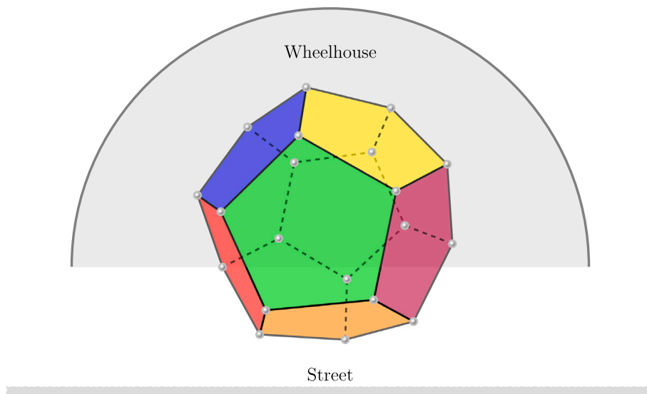
Fig. 14. Schematic of the volume source and its position in the measurement set-up.
