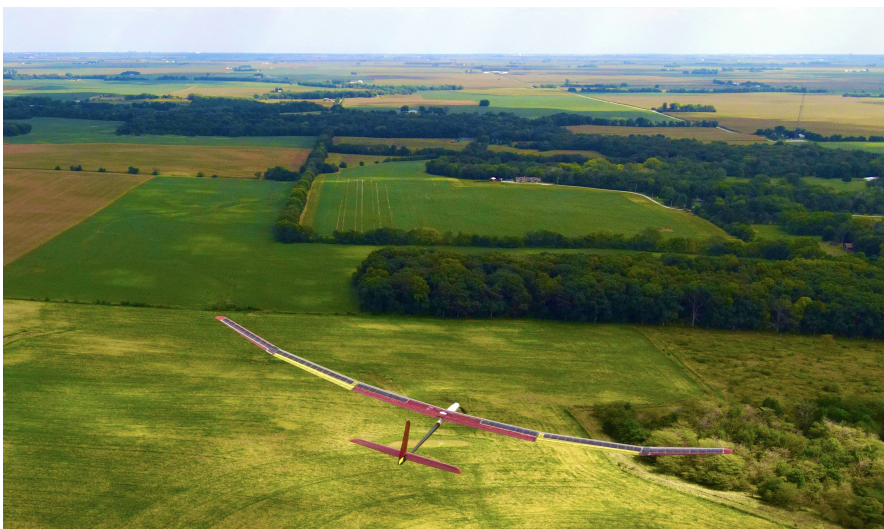
Figure 1.1: The UIUC-TUM Solar Flyer aircraft equipped with solar panels flying autonomously in an agricultural environment [22].
