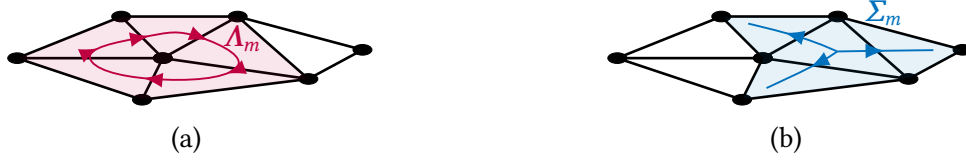
Fig. 3.4: Examples of loop-star basis functions: (a) RWG loop formed around a vertex by five RWG functions; (b) RWG star formed around a triangle by three RWG functions.
