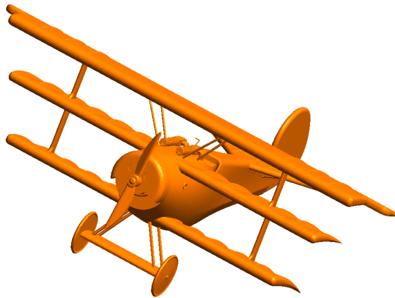
Fig. 4.14: Model of a Fokker Dr.I with an approximate wingspan of 7 m containing N_H = 390 global loops. The model is discretized with 196 280 triangles and 294 420 RWGs. © 2023 IEEE
