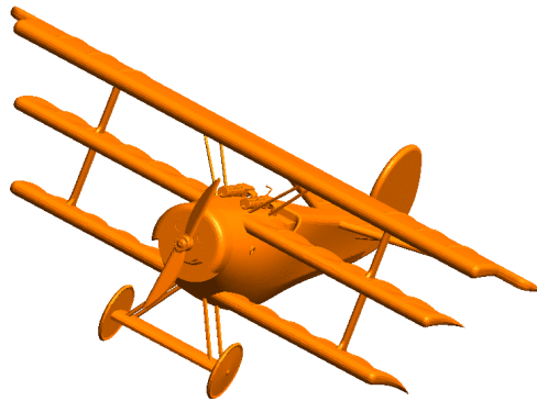
Fig. 5.10: Model of a Fokker Dr.I with an approximate wingspan of 7 m. The model is discretized with 196 280 triangles and 294 420 RWGs. © 2023 IEEE
