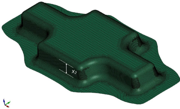
Fig. 2 Exemplary geometry of the cross-die component studied here. The definition of slant depth is indicated in white, i.e., design variable x_2 , used here
