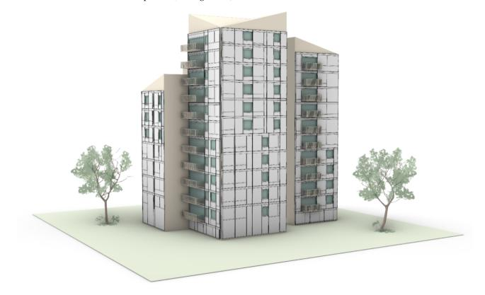
Figure 13. Building model and detailed prefabricated module layout of the demo-building in Milan.
