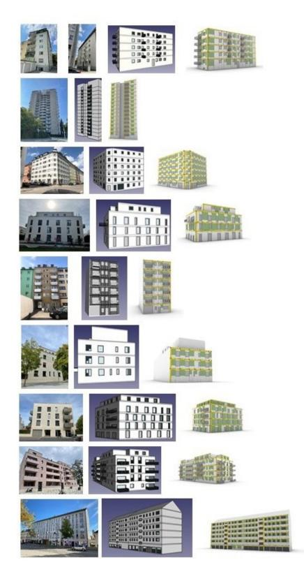
**Figure 14.** Residential buildings where the tools were applied. In the columns in the left and center, the initial inputs are shown, that is images of the building and the building models. In the column in the right, the building models with the prefabricated module layouts are shown, that is, the output of RG1.2 and RG1.4.
