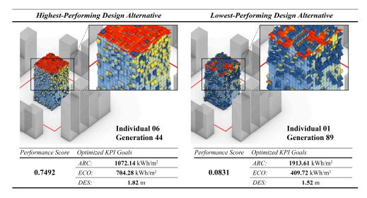
**Figure 6.** Comparison between the highest- and lowest-performing optimized design alternatives. Solar radiation values are depicted from the lowest (blue) to the highest (red) values. The figures were previously published in (Selvan et al. 2023) [69].
