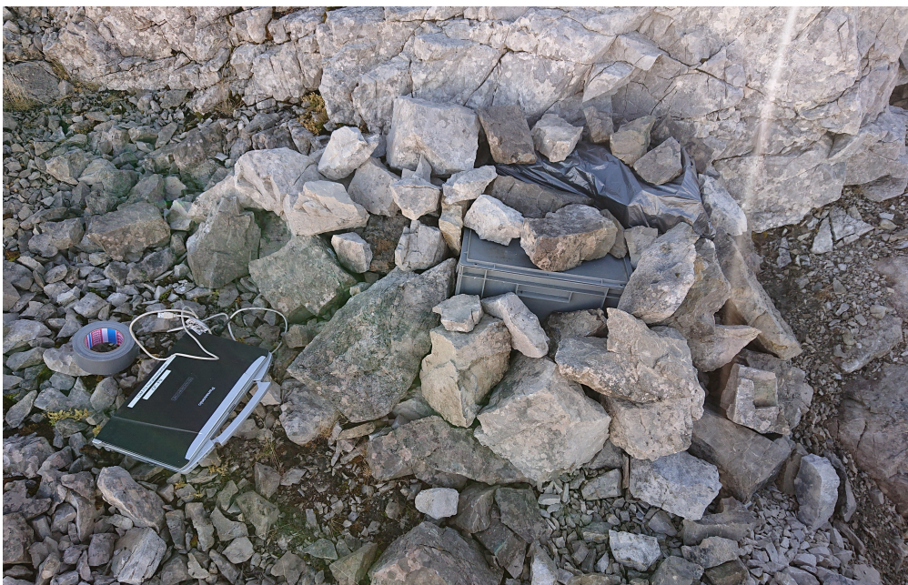
Supplementary Fig. A.1.5: Photo of seismic station SA22 during maintenance. During operation, the station is completely covered with rocks to protect the geophone from wind and rain.
