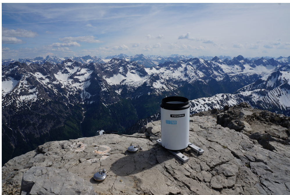
Supplementary Fig. A.1.3: Photo of tipping bucket rain gauge on the summit of Hochvogel.
