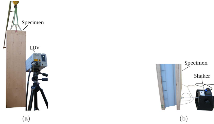
Figure 5. Scan setup using heavy-duty slings for suspension with Laser Doppler Vibrometer (LDV) (a) and shaker (b).
