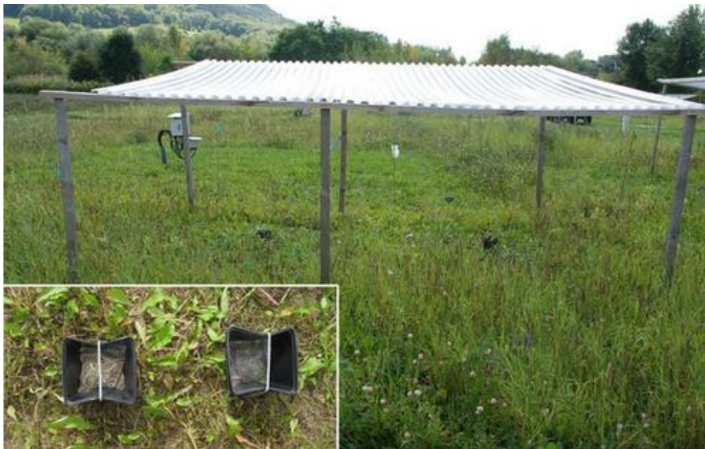
Figure 5: PVC rain shelters utilized to simulate drought during summer months for our field experiment. In the top left corner the litter decomposition unit utilized during the study where soil samples were extracted from are displayed (adapted from Vogel et. al 2013).
