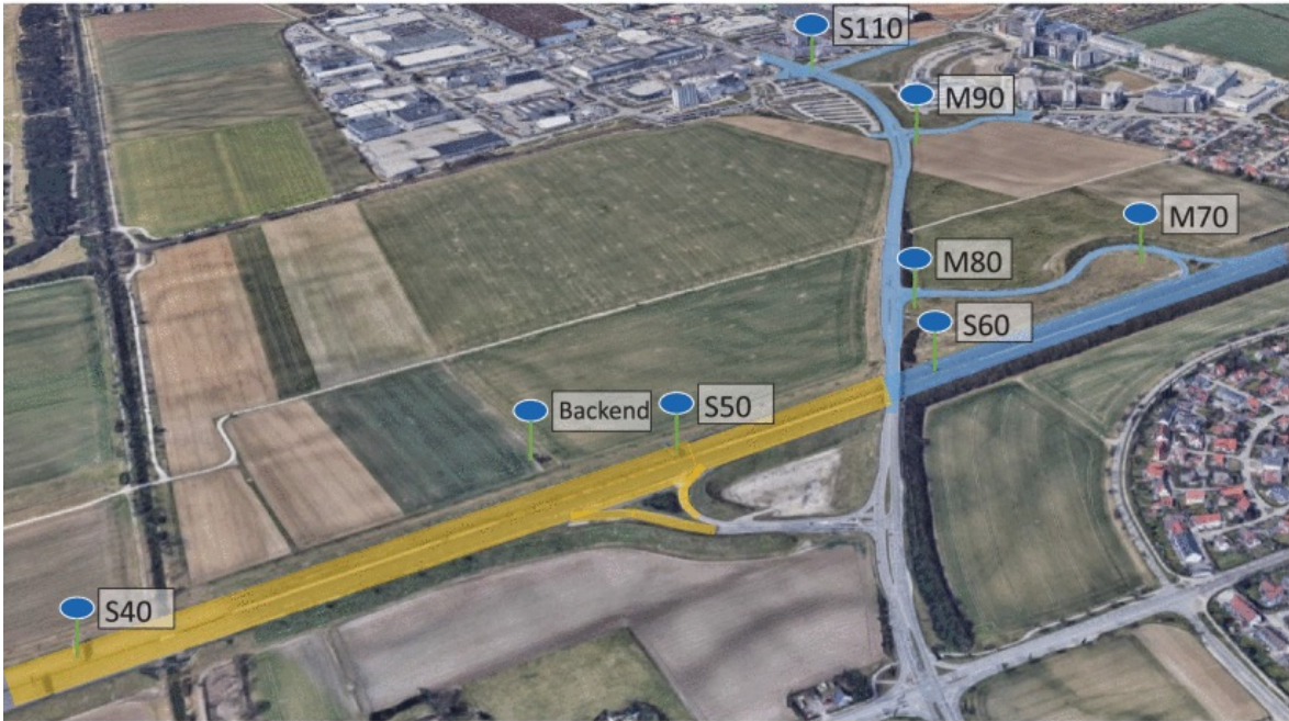
Figure 1.1: Overview of the test bed Providentia++ taken from [Cre+22]. This test bed spans the autobahn A9 and the highway B471 near Munich, covering a total length of 3.5 km
