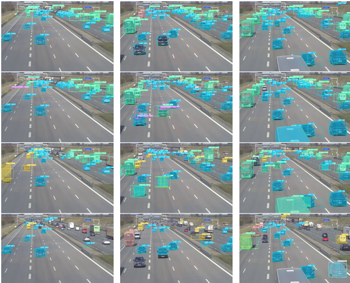
Figure 6.2: Highway: Qualitative comparisons on one high way sequence. Baseline detector YOLOv7_coco (first row) and the proposed detector with model weight YOLOv8_coco (second row), YOLOv8_tumtraf (third row) and with model weight YOLOv8_coco_tumtraf_1920 (fourth row).The visualizations include 2D bounding boxes, 2D masks, 3D bounding boxes, and category labels.
