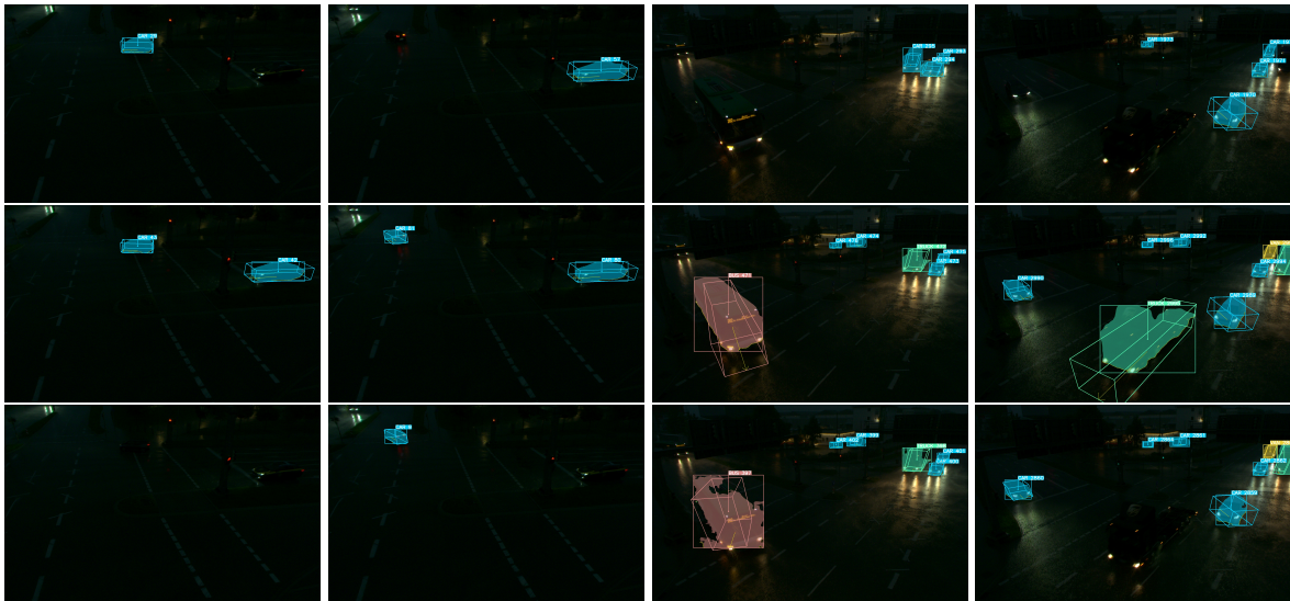
Figure 6.1: Night sequence: Qualitative comparisons of night sequence prediction of baseline detector YOLOv7_coco (first row) and the proposed detector with model weight YOLOv8x_tumtraf (second row) and with model weight YOLOv8x_coco_tumtraf_1920 (third row). The visualizations include 2D bounding boxes, 2D masks, 3D bounding boxes, and category labels.
