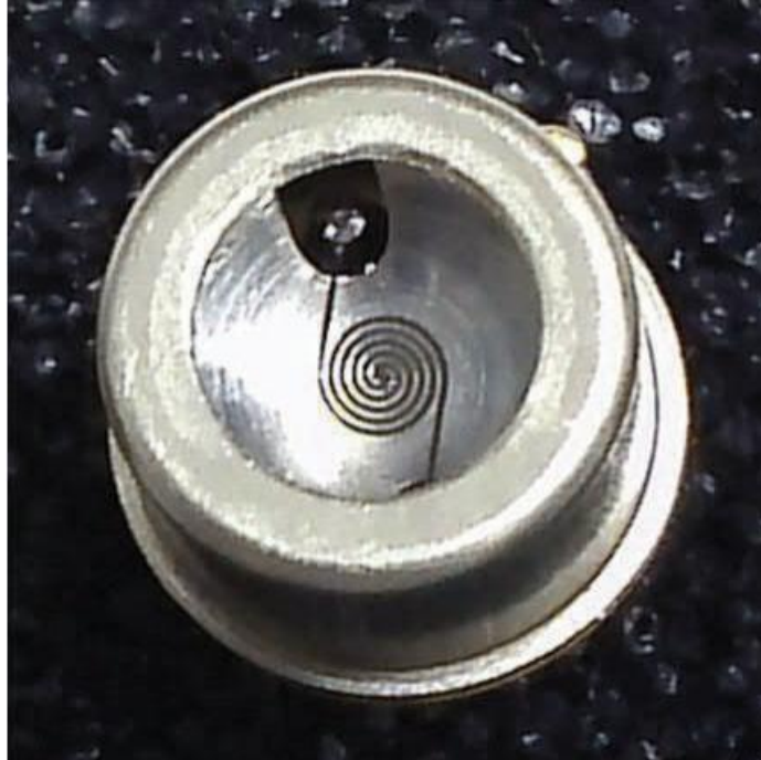
Figure 6: Thermal IR emitter with a spiral shape radiation element ( 2.8 \text{ mm}^2 ) with an NiCr nanostructured layer, operating with a near-blackbody characteristic (Schossig et al., 2015)
