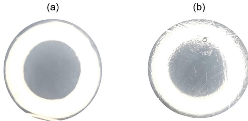
Fig. 10. Visual comparison of a transparent polypropylene tray under a ring-shaped light: (a) regular reference and (b) polymer with a stronger scattering optical structure.
