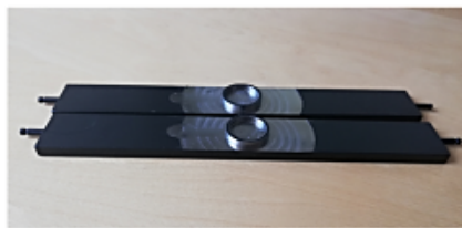
Fig. 3. Sealing jaw for the annular heat-sealing with a Teflon-coated sealing surface.
