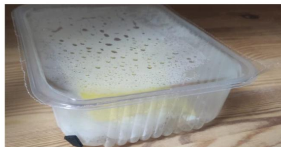
Fig. 5. Packaging with adjusted relative humidity of 100% to evaluate the influence of H 2 O condensation within a package on the measurement accuracy of the demonstrator.
