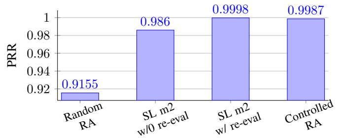
Fig. 2. Comparison of different sidelink resource allocation modes.
