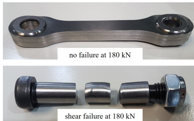
Figure 2.17: Tension-torsion strap and 12 mm attachment bolt after tensile strength test, actual UL 180 kN
