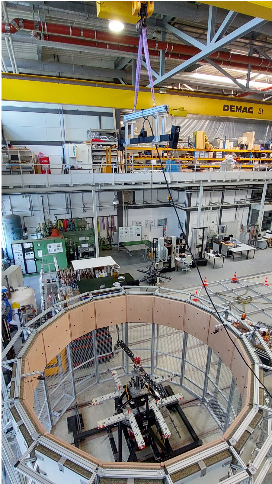
Figure 3.10: Photogrammetry measurement setup of the ARAMIS SRX 1600 MV4200 HD sensor attached to the lab crane 4.365 m above the MERIT rotor plane
