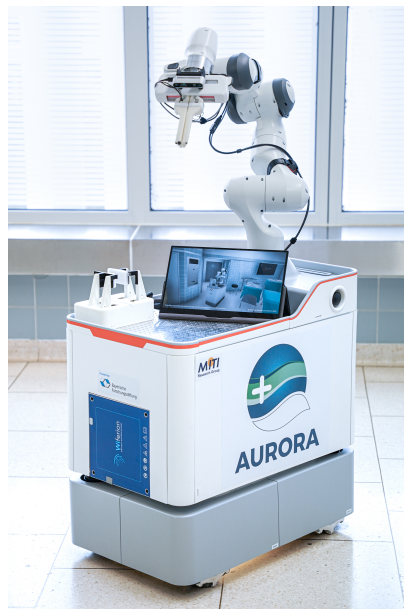
Figure 2.2: The AURORA prototype features a mobile omnidirectional base platform equipped with a robotic manipulator arm. A custom-designed endeffector and an auxiliary mechatronic module enable the robot to open sterilely packaged surgical materials.
