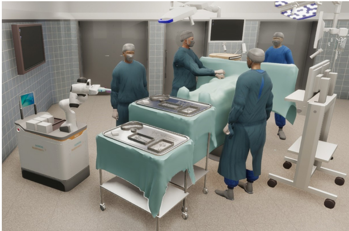
Figure 1.2: A conceptual rendering of the AURORA robot (left side) within the OR environment is shown. AURORA supports the surgical team by providing surgical materials and adjusting devices in the immediate surroundings.
