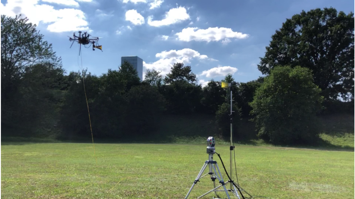
Figure 5.5: Picture of the cylindrical measurement setup. The laser tracker was placed under the AUT, maintaining a stable line-of-sight to the reflector target underneath the field probe at the front of the UAV.
