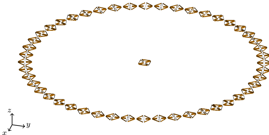
Figure 8.3: Simulation model of a DVOR. All antennas are similar ALAs, where the antenna ring consists of 48 elements, which are rotated such that always the same edge points to the center of the ring.
