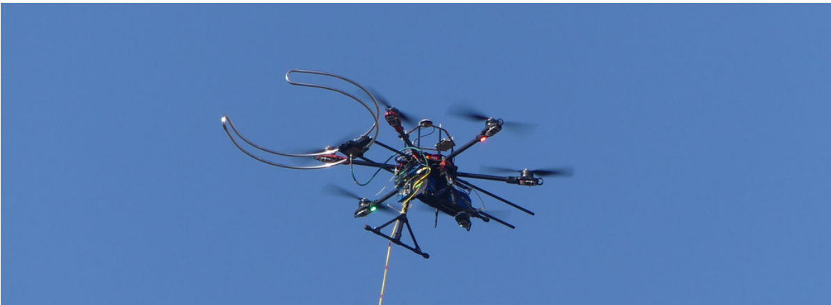
Figure 8.15: UAV including field probe during a measurement flight. A ring dipole antenna served as field probe which was mounted to the front of the UAV, even in front of the front motors.
