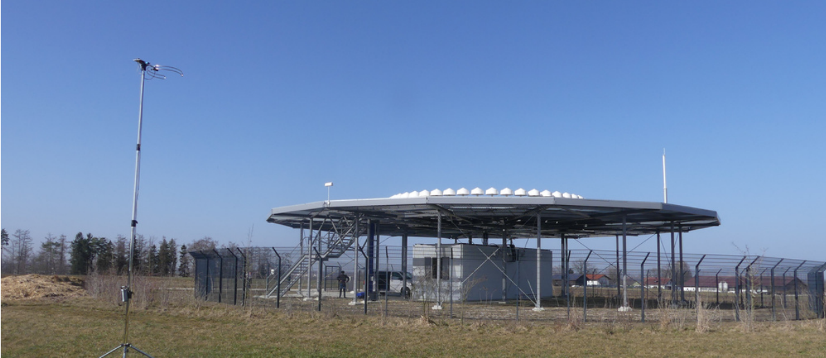
Figure 8.14: Picture of the DVOR Ottersberg where the counterweight or artificial ground plane is prominently visible. The reference antenna is also depicted which was mounted on a stand and served as phase reference for the measurements.
