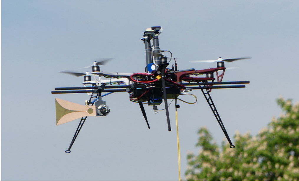
Figure 4.2: Hexacopter during measurement flight with vertically polarized field probe mounted at the front. The prism reflector target is placed at the front of the UAV and next to the probe antenna where a stable line-of-sight to the laser tracker can be ensured. Also, the optical fiber that connects the UAV with the ground in terms of control and RF signals is visible.
