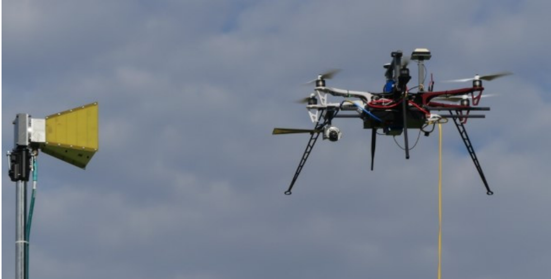
Figure 5.1: Picture of the AUT and the UAV during the planar in-situ measurement. The horizontally polarized field probe is depicted which is connected to the measurement receiver at the ground via an RF-over-fiber link.
