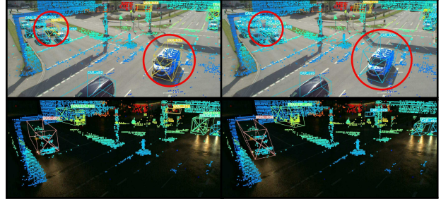
Figure 8. Qualitative results of our CoopDet3D (left) and the InfraDet3D (right) model on the TUMTraf Intersection test set during day and nighttime. Detected objects marked with a red circle were classified correctly by CoopDet3D.
