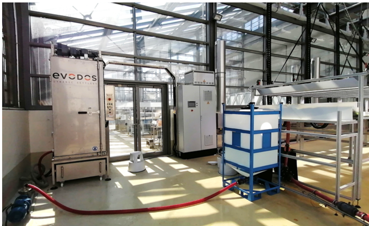
Figure 4.9: Exterior view of Evodos™ centrifuge connected to the pilot-scale TLC photobioreactor. Microalgae suspension pumped into the collection tank continuously is fed to the centrifuge using the associated progressing cavity pump located on the floor to the left of the centrifuge compartment. The control cabinet with a touch screen display panel is located on the right side of the hall door.
