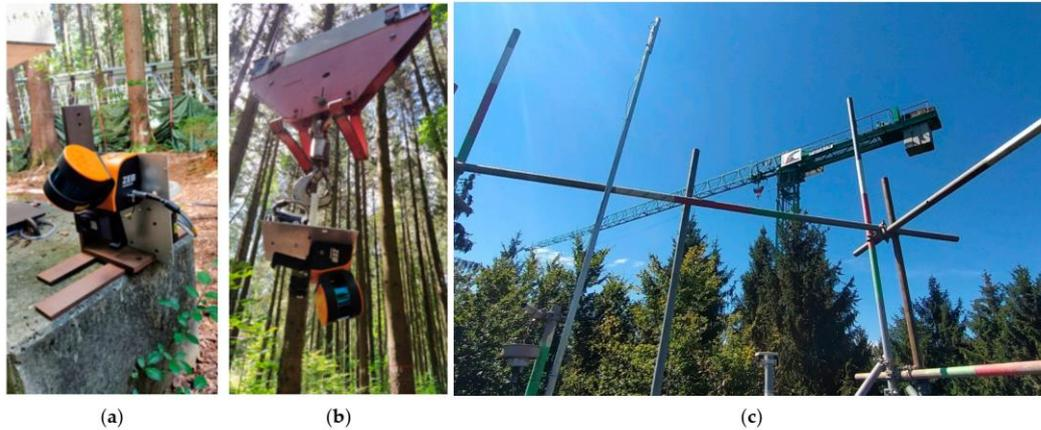
**Figure 1.** The mobile laser scanner in the start position (a) and attached to the crane (b). During operation, it was lifted over the canopy and moved smoothly over the canopy of the forest stand. Figure (c) shows the crane itself.
