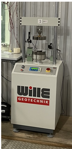
(c) Load frame for performing the uniaxial compression and creep tests within a chamber of controlled temperature and humidity.
