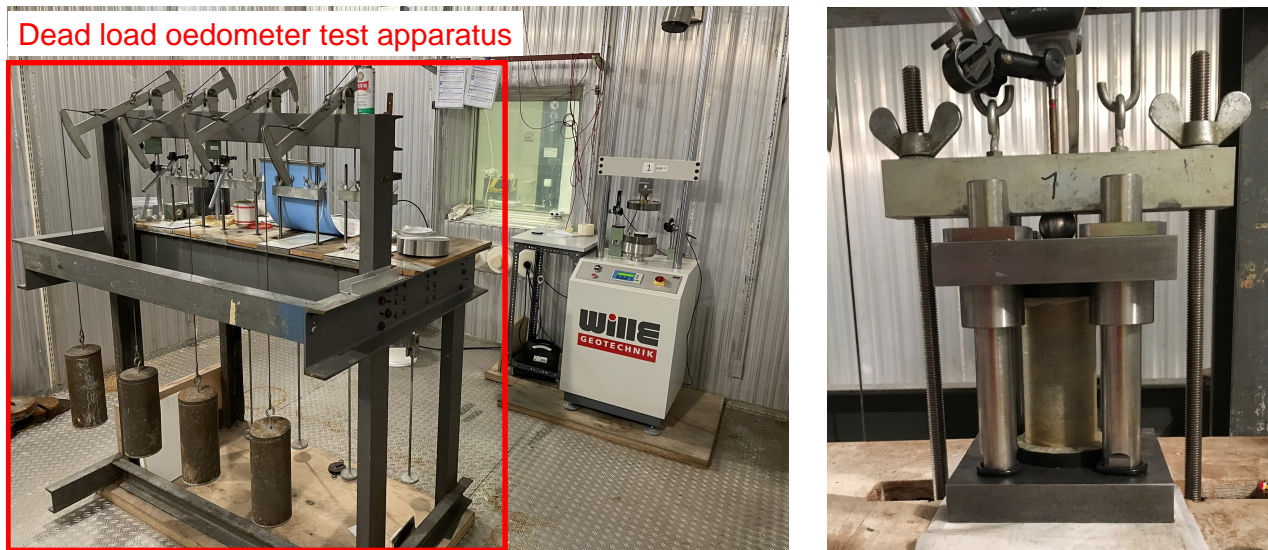
(a) Dead load oedometer test apparatus in the cooling chamber. (b) Test setup for the dead load oedometer apparatus.
