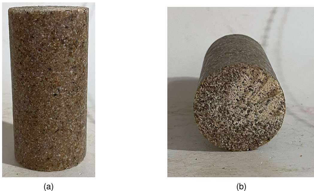
Figure 3.8.: Example of a prepared frozen Karlsruhe sand sample with a diameter of about 50 mm and a height of about 100 mm after freezing and before testing.
