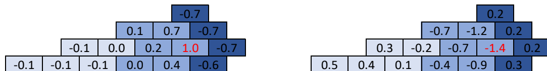
Figure 4: Deviations (%) from the reference of the normalized neutron flux distributions for the SP 3 solvers of FENNECS (left) and DYN3D (right) with 96 radial elements per assembly. The red numbers are the maximum deviations.
