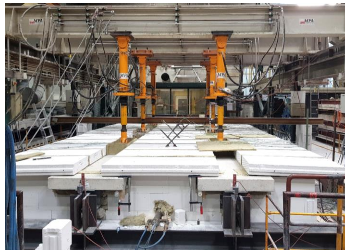
Figure 7: Large-scale fire test setup: furnace and composite beams
