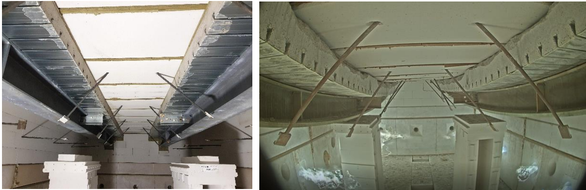
Figure 8: Composite beams before and during fire test
