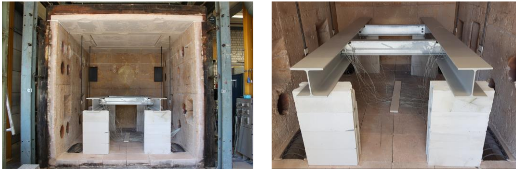
Figure 4: Position of the beams in the furnace
