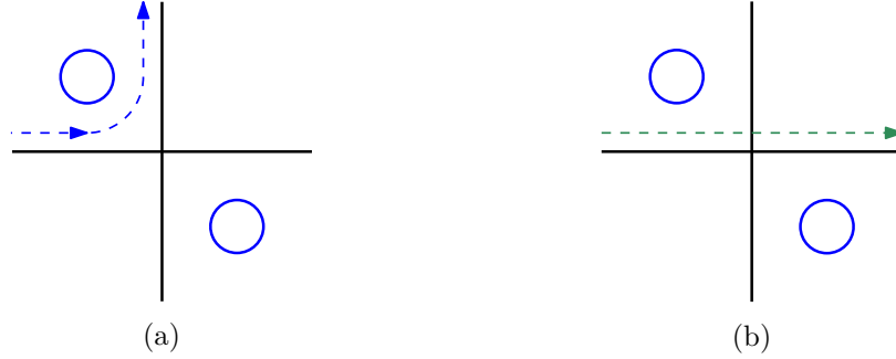
Figure 6.20.: Crosstalk from left. (a) A resonant crosstalk from left drops to up, suffering a drop loss. (b) A nonresonant crosstalk from left travels to right, suffering a passing loss, a crossing loss and a passing loss.
