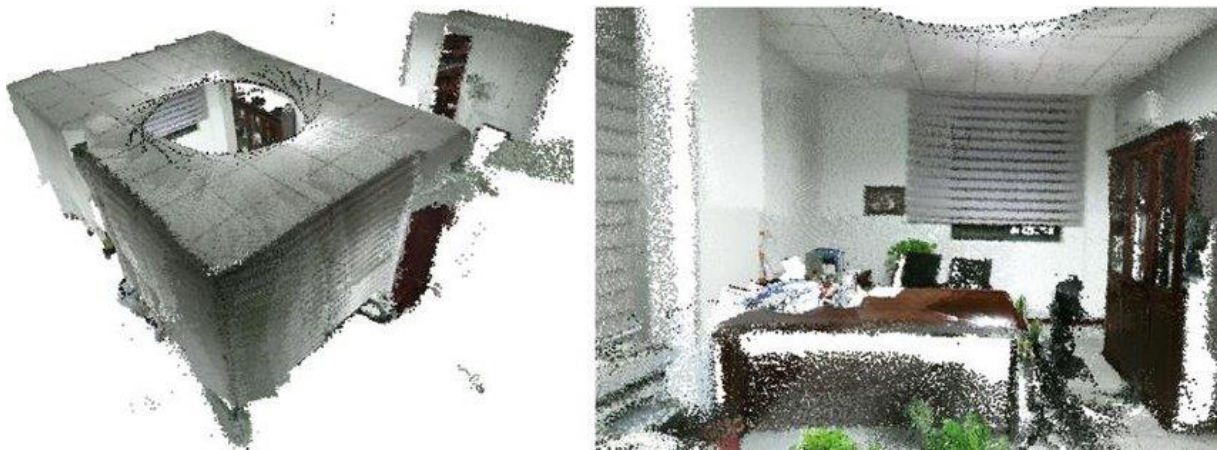
Figure 2. 10: Point cloud captured by RGB-D camera in typical indoor scenes (Chen et al., 2018)
