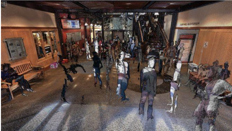
Figure 2. 9: Dense TLS indoor point cloud of a building at Oregon State University (Person et al., 2022)
