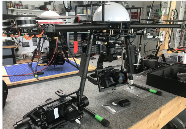
Fig. 2 UAV with Sigma camera (foreground, left) and Sony a7R (mounted in gimbal)
