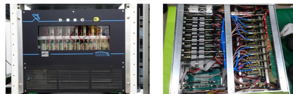
Fig. 4 (Left) Front view of the DBBC3 newly installed at the Ishioka station. (Right) Top-down view.
