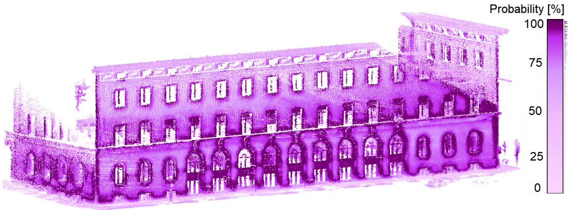
Figure 4.14 Exemplary results of the modified network: point cloud colors according to the probability vector of the class window .
