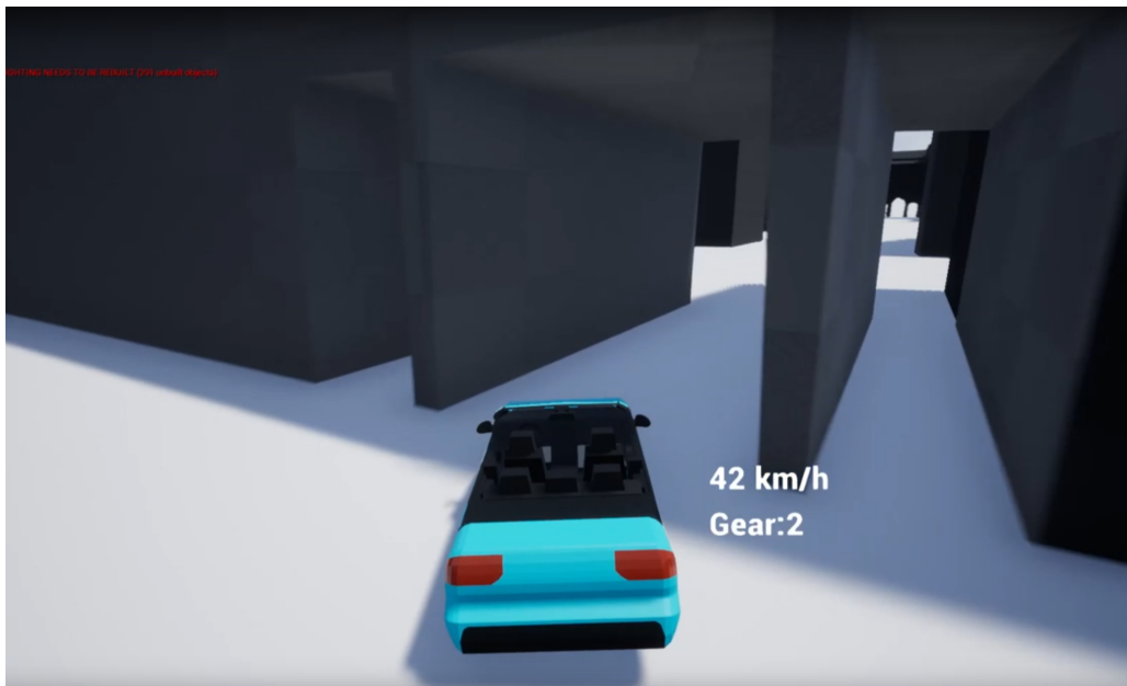
Figure 8.3 A screenshot from an Unreal Engine application showcasing usage of enriched models as a virtual testbed for testing car navigation systems: The LoD3 model with underpass mimics the real situation and enables drive through the building, impossible in footprint-extruded LoD2 or LoD1.
