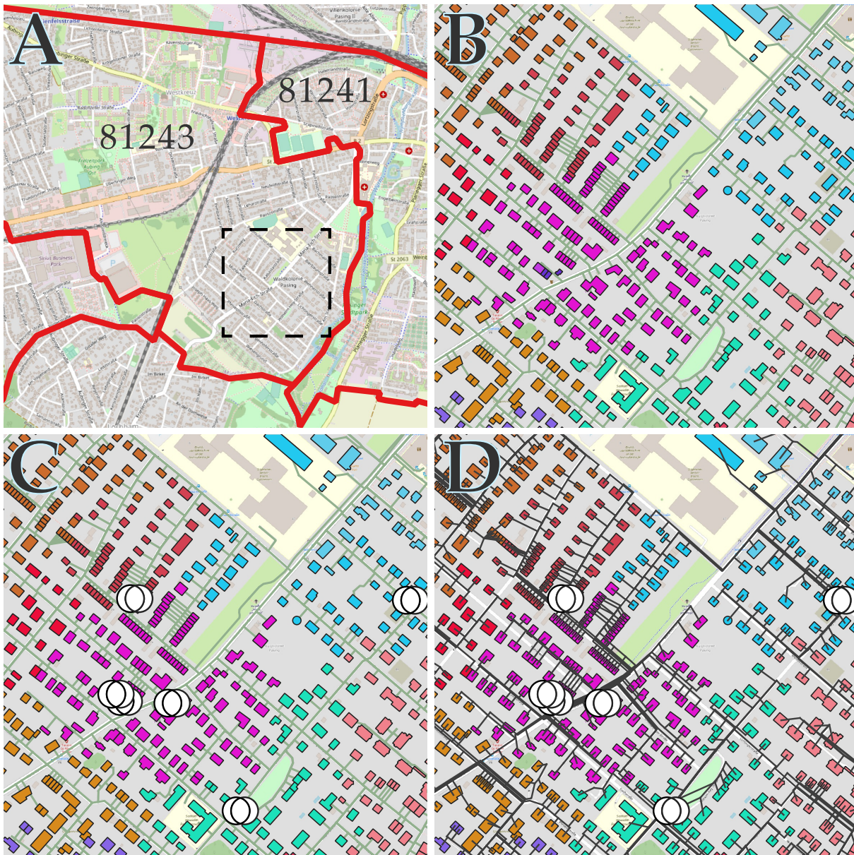
Figure 3.24: The pylovo workflow illustrated in multiple steps. A: postcode area selection, B: building clustering, C: transformer positioning, D: topology generation and cable dimensioning.
