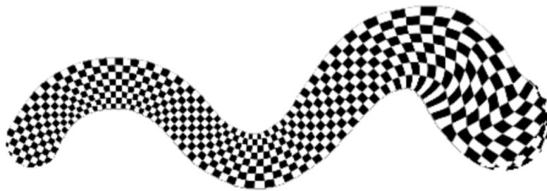
Figure 5.11: Interruption of pixel averaging when the drawing stops.
